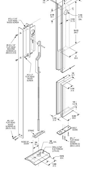
Basic lock mechanism boxed with actuator arm attached, rod/bolt assembly unattached. Stainless steel bolt guide, mounting screws and installation instructions included. Cylinders available at extra cost. Shipping weight: 1-1/4 lbs.
